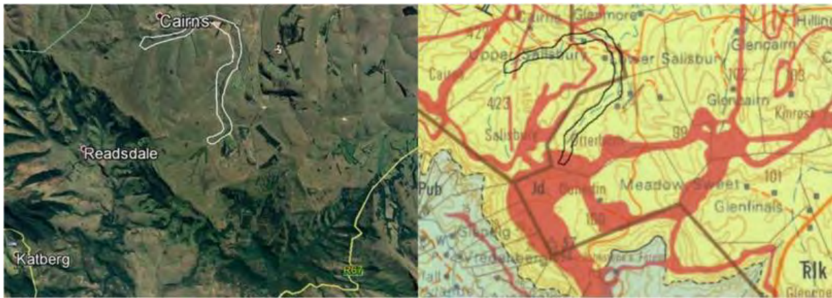
Figure A The wetlands identified in the polygon below in a Google Earth Image on the left and the geology Map (Council for Geoscience) on the right. The Tarkastad formation is the yellow colour and the dolerite intrusions in red (Source: Dr Piet-Louis Grundling)
