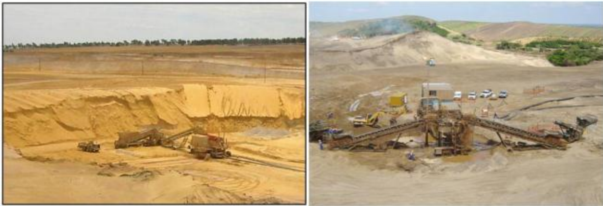
Plate 2.1: Typical loader and hopper dry mining operation
