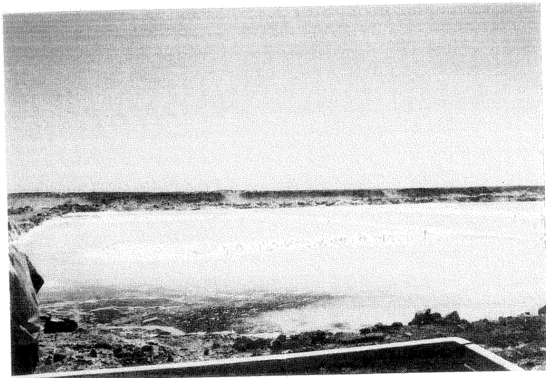
Figure 2. Brine is pumped unto hardened surface where evaporation and crystal growth ensues.
