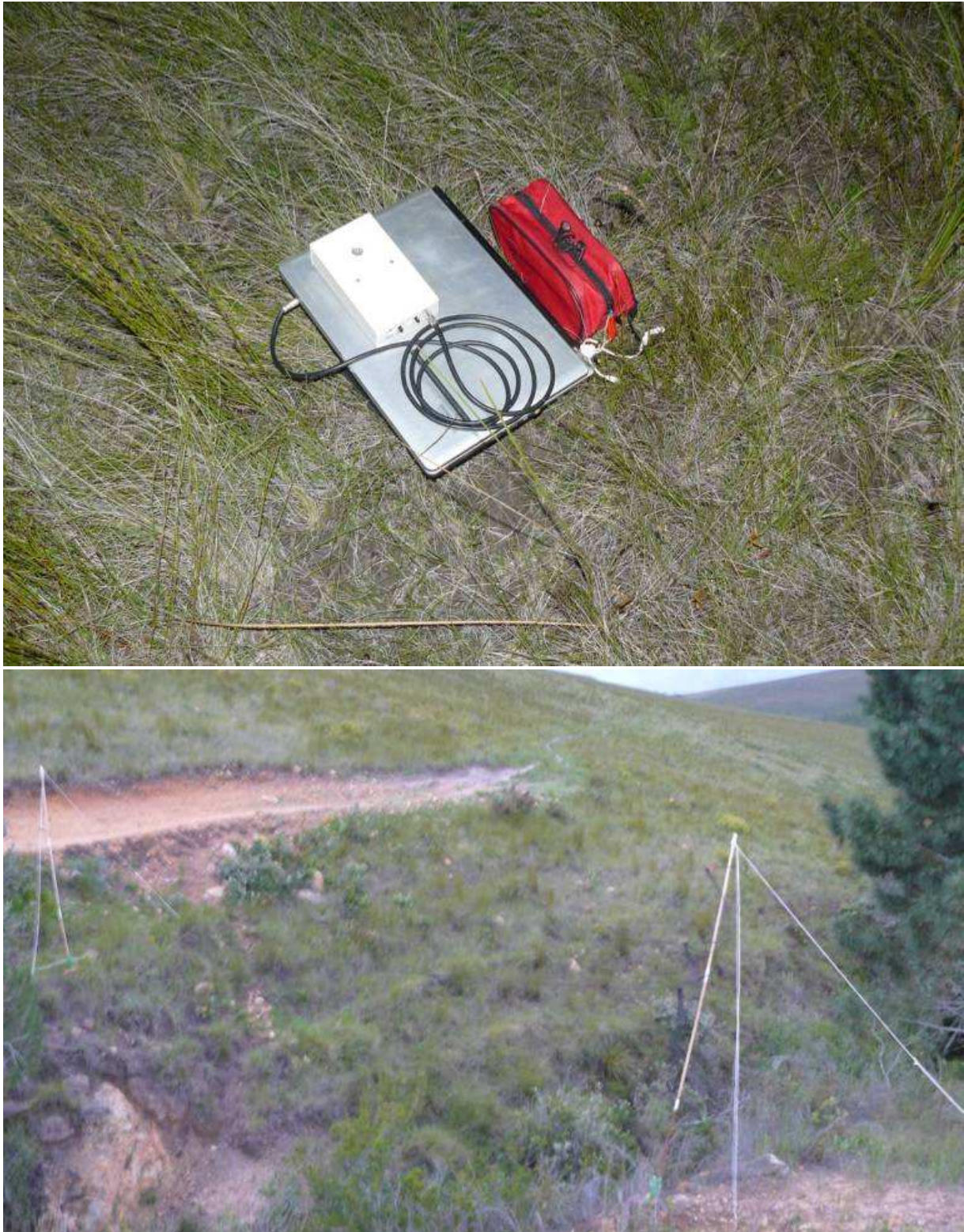
Figure 6: (top) The time expansion type bat detector (BD3) set up with a field laptop and external long life battery to passively record bat echolocation calls; (bottom) a mist net set up across a drainage gully (MN3) where habitual bat flight is possible, the actual fine net is between the two poles and not visible in this photograph.
