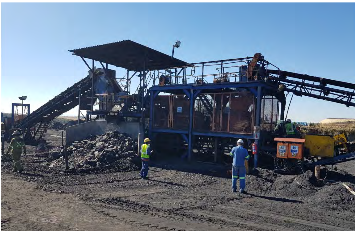
FIGURE 2-3: EXAMPLE OF A TYPICAL WASH PLANT
