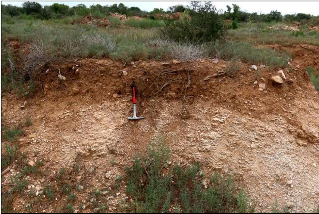
Figure 17: Well-developed calccrete hardpan beneath gravelly brown soils exposed in a shallow quarry area in the south-eastern sector of the project area (hammer = 30 cm).
