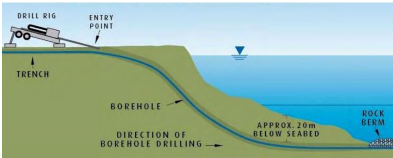
Figure 3.18: Schematic presentation of horizontal directional drilling method.
