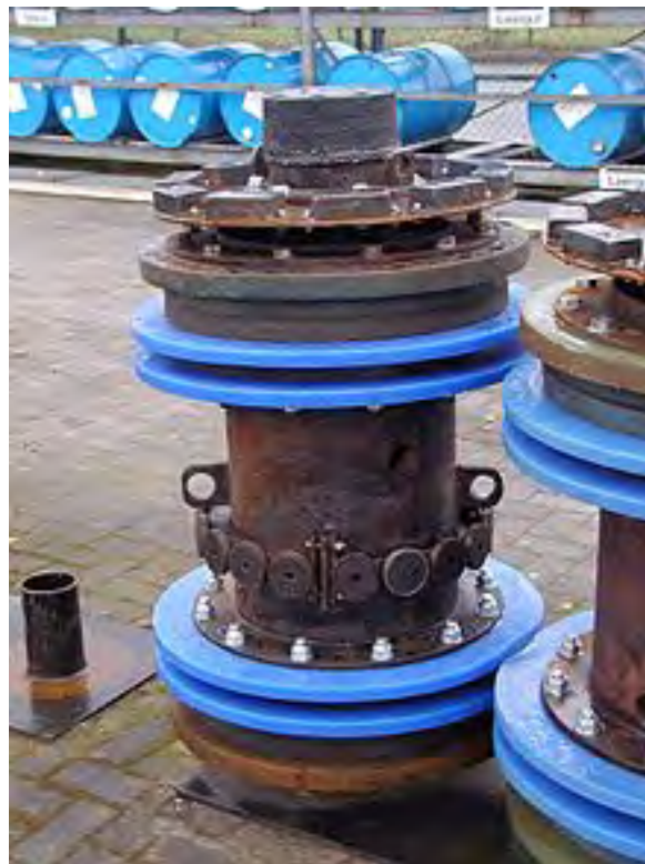
Plate 3.14: An example of a cleaning pig for a 28-inch oil pipeline ( https://en.wikipedia.org/wiki/Pigging ).
