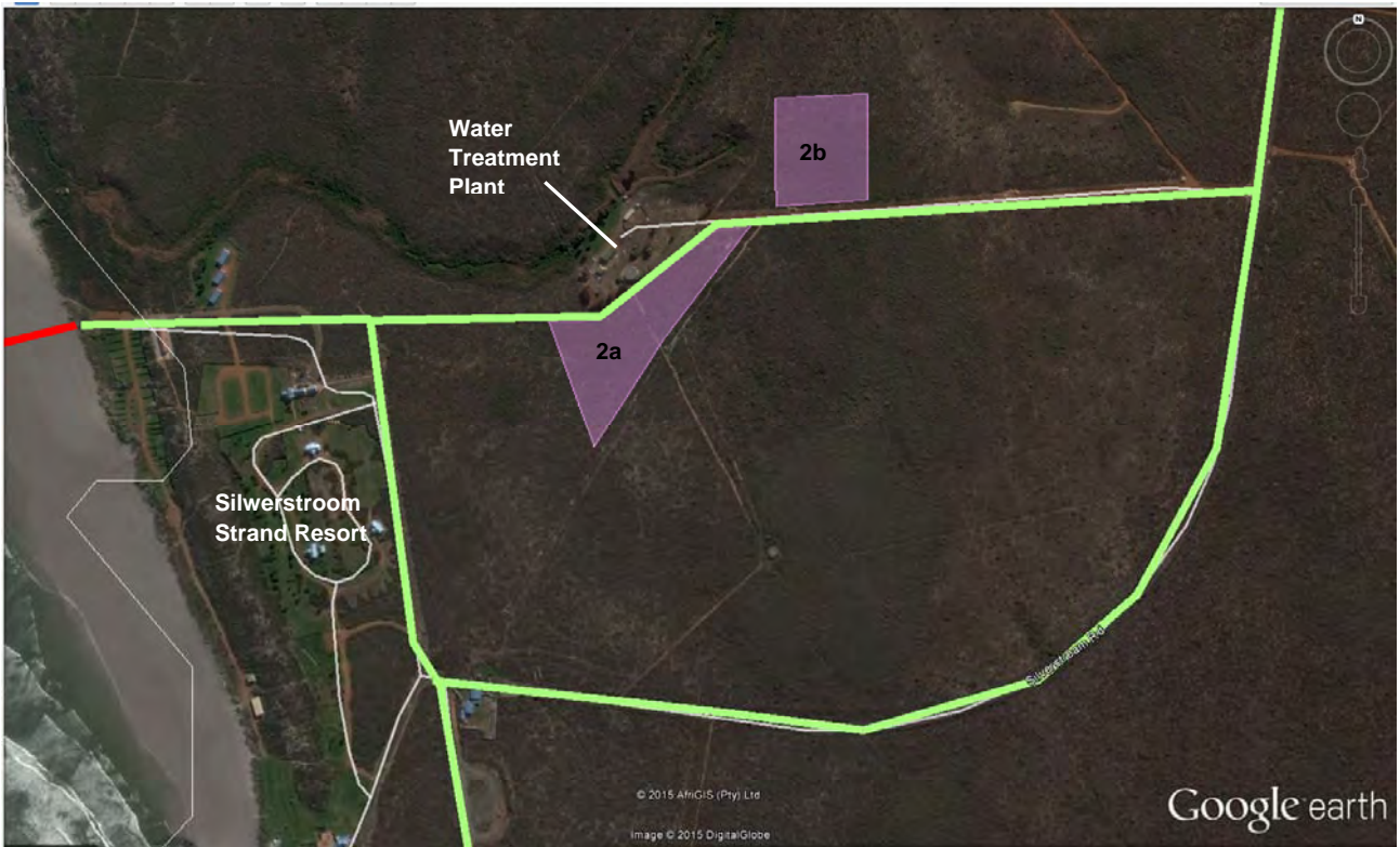
Figure 3.14: Location alternatives (Alternative 2a and 2b) for the proposed onshore gas receiving facility near the existing Silwerstroom Strand Water Treatment Plant (after GoogleEarth 2015). The proposed onshore pipeline alternatives associated with the Silwerstroom Strand shore-crossing are also shown.
