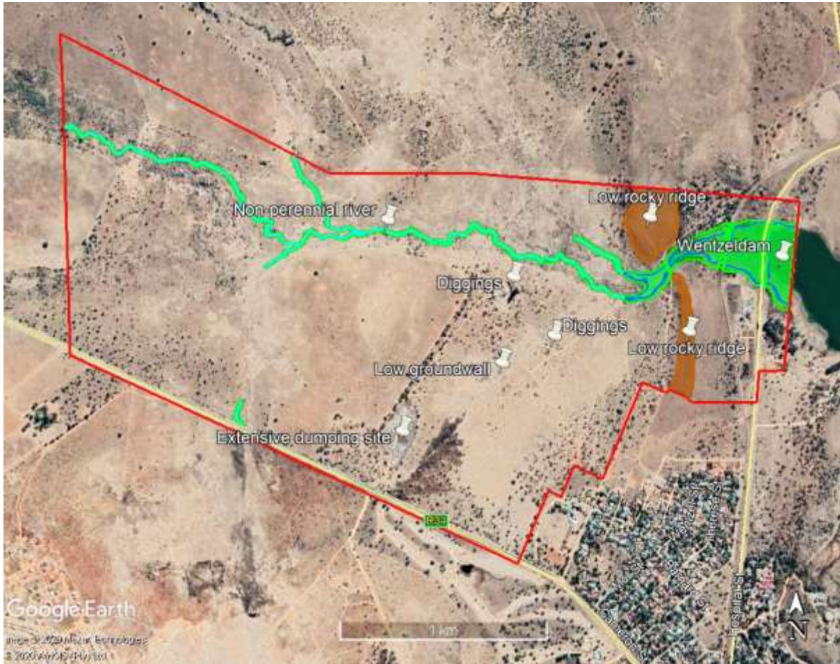
Figure 4 Indication of non-perennial river (active channel, riparian zone, buffer zone), in-channel dam and low rocky ridges at the site.
