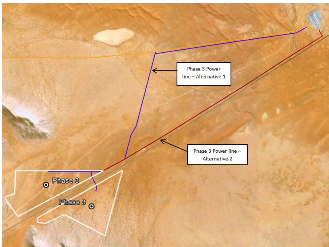
Figure 10.2: Grid Connection Routing Alternatives – Phase 3
