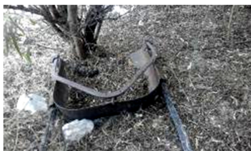
Figs. 38 and 39. The corrugated iron building that was erected over the old well. Adjacent to this building hidden under the vegetation is an implement that in Afrikaans is known as a “damskrop”. (Earth-scoop.) Basically it is a scoop drawn by draft animal used to shift soil for an array of purposes. (Photos S.M. Miller 2018.)
