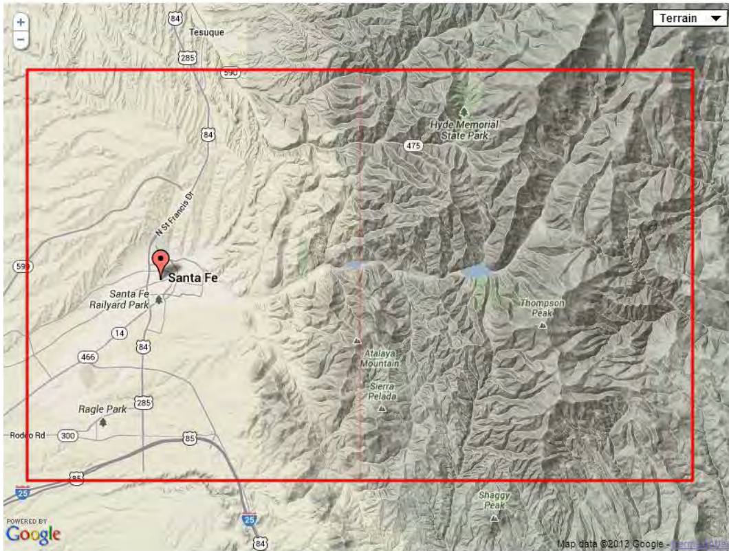
Figure 1: Two \frac{1}{8} degree grid cells (note the lighter red vertical line that bisects the heavier red rectangle) that define the climatic conditions for the City of Santa Fe (left) and the Santa Fe River reservoirs (right). Nichols Reservoir, which is the smaller of the two blue water bodies visible actually straddles the cells, while McClure is centrally located in the more easterly cell. Image from http://gdo-dcp.ucllnl.org/downscaled_cmip_projections/dcpInterface.html#Projections:%20Subset%20Request
