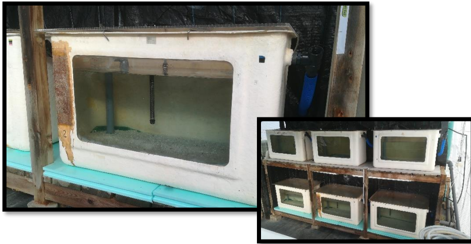
Figure 2.3.1. Illustrative representation of the experimental setup comprised of six 250L tanks fitted with bottom filters. The tanks were placed in a man-shift dark room and lights were installed directly above each tank to simulate summer light conditions in shallow waters and facilitate video recordings from underwater and external cameras.
