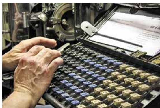
The keyboards of line casting machines are arranged according to the letters that are used most often in typing text.
