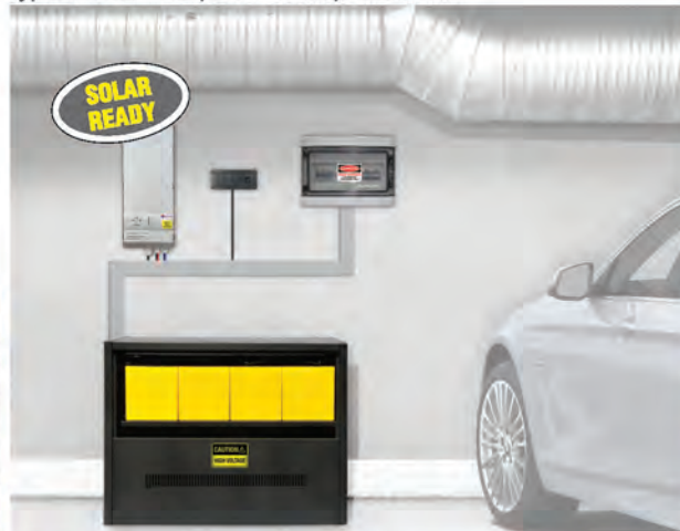
Typical residential power backup installation
