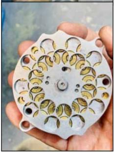
ST MACHINING LOADING BLOCK, OPEN. IF THE ROUND GOES ALL THE WAY IN SMOOTHLY AND WITHOUT RESISTANCE, IT HAS A GOOD CRIMP, A FLAT RIM, AND NO SPLITS. THE ONLY THING IT WON'T CATCH IS A CANNELURE, WHICH CAN CAUSE A CASE SEPARATION, LOCKING UP YOUN RIFLE. CLOSING IT CHECKS ROUNDS FOR HIGH PRIMERS. MERNICKLE HOLSTER'S MAKES A POUCH FOR THEM. I HAVE SEEN THEM WITH ANTLERS TIED TO ONE OF THE OUTSIDE HOLES, THEN HUNG FROM A GUN BELT.
