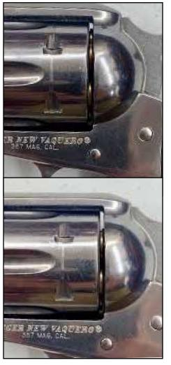
ROUND UNDER HAMMER (TOP). NO ROUND UNDER HAMMER, CORRECTLY LOADED (BOTTOM).
