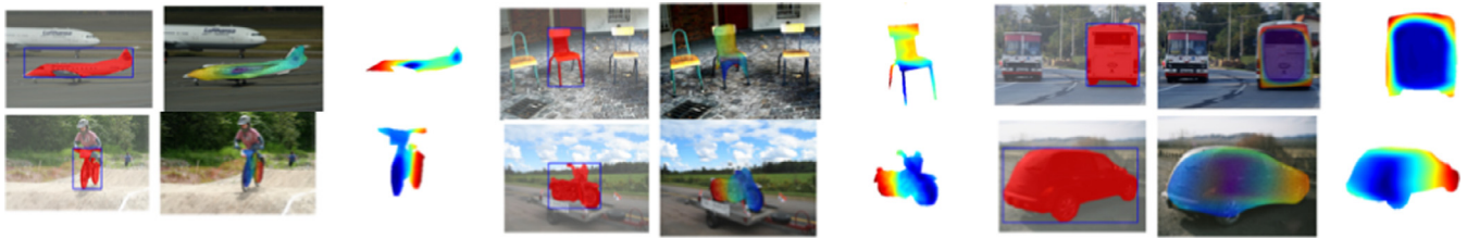
Fig. 20. Fully automatic reconstructions obtained from just a single image using our system described above. Each panel (from left to right) shows the image with automatic detection and segmentation, the 3D model inferred using our method ‘replaced in place’ and the final depth map obtained.
