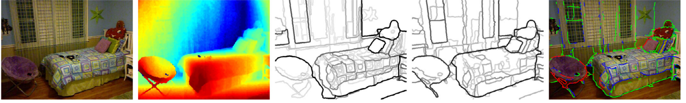
Fig. 14. Contour detection: color image, depth image, contours from colour and depth image, contour labels. (For interpretation of the references to color in this figure text, the reader is referred to the web version of this article.)
