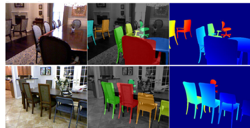
Fig. 19. Model placement: color image, placed models projected onto color image, depth map of rendered models (blue is closer, red is farther away). (For interpretation of the references to color in this figure legend, the reader is referred to the web version of this article.)
