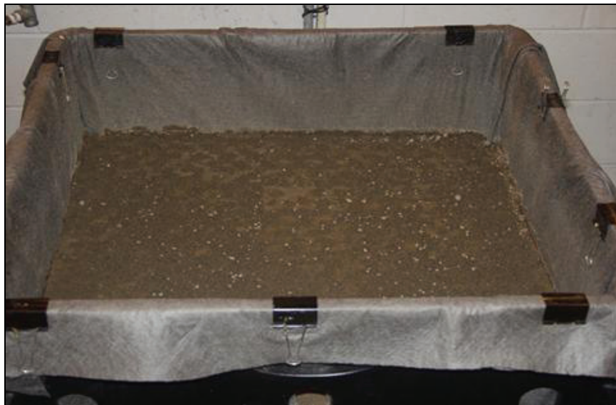
Figure 5. Loaded lysimeter showing soil surface.
