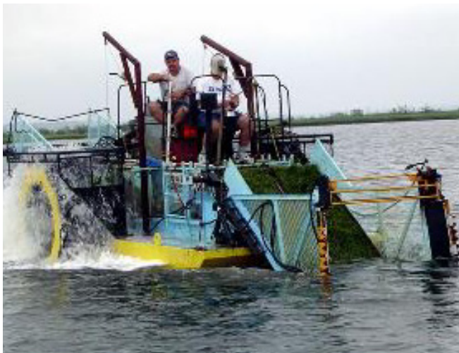
Figure 3. Commercial aquatic vegetation harvester used for the collection of eelgrass reproductive shoots (photo by VIMS).
