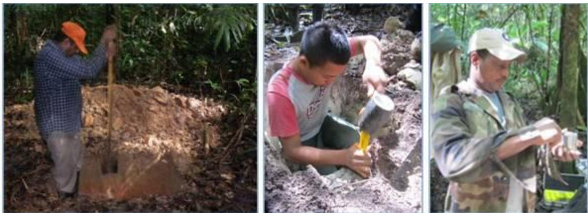
Figure 14 Sampling SOC. From left to right: Digging a pit of 100 cm x 50 cm to a depth of 100cm - sampling at different depths- preparing the sampling rings for transport
