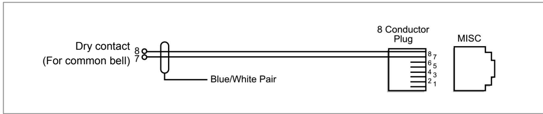
Figure 7.19 Connecting Common Bells
