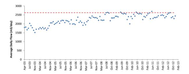
Figure 3.19. Monthly trends in the volume of effluent released from the Saldanha WWTW, Apr 2003-December 2012, and authorised total volume per year expressed as a daily limit (red line). Allowable discharge limits as specified in terms of the exemption issued by DWAF under the National Water Act 1998 are represented by the dashed red line.
