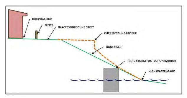
Figure 5.12 Submerged storm protection barrier proposed for Leentjiesklip Caravan Park (Common Ground Consulting 2013b).
