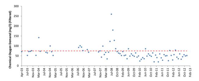
Figure 3.22. Monthly trends in the numbers of Chemical Oxygen Demand in effluent released from the Saldanha WWTW, April 2003 - December 2012. Allowable limits as specified in terms of a General Authorisation under the National Water Act 1998 are represented by the red line.
