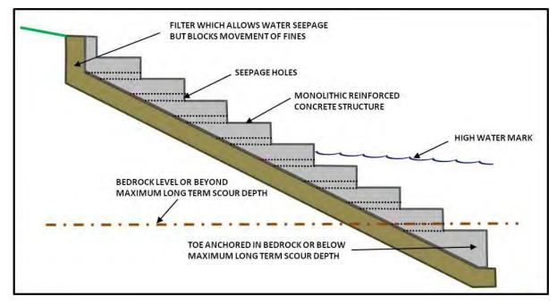
Figure 5.14. Design proposal 2 for the proposed Melck Street walkway: Concrete steps. Source: Common Ground Consulting (2013b).
