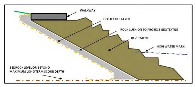
Figure 5.15. Design proposal 3 for the proposed Melck Street walkway: Rock revetment. Source: Common Ground Consulting (2013b).
