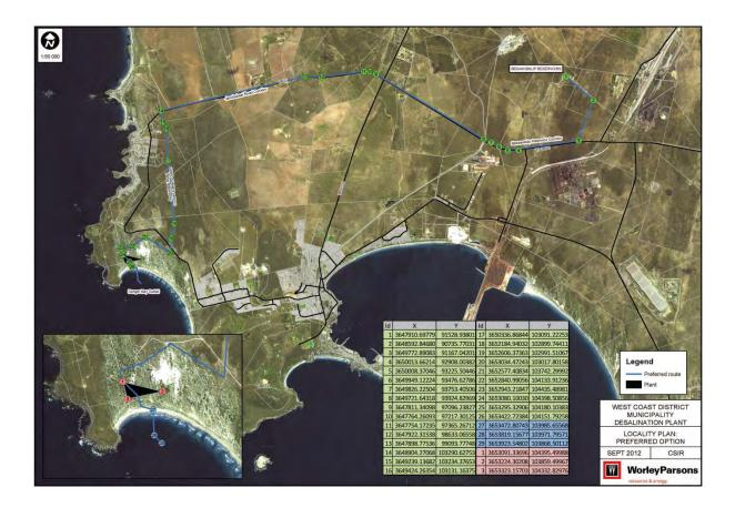
Figure 3.17 Map showing preferred location of intake and discharge points for the WCDM desalination plant. Source: CSIR 2013.
