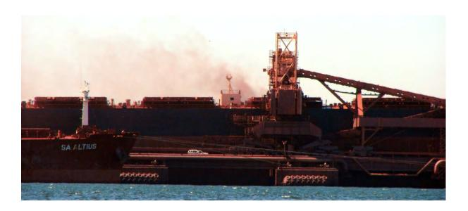
Figure 3.16 An iron ore vessel being loaded showing associated iron ore dust emission. Freshwater from the Transnet RO plant will be used to mitigate this impact by wetting the ore before loading.
