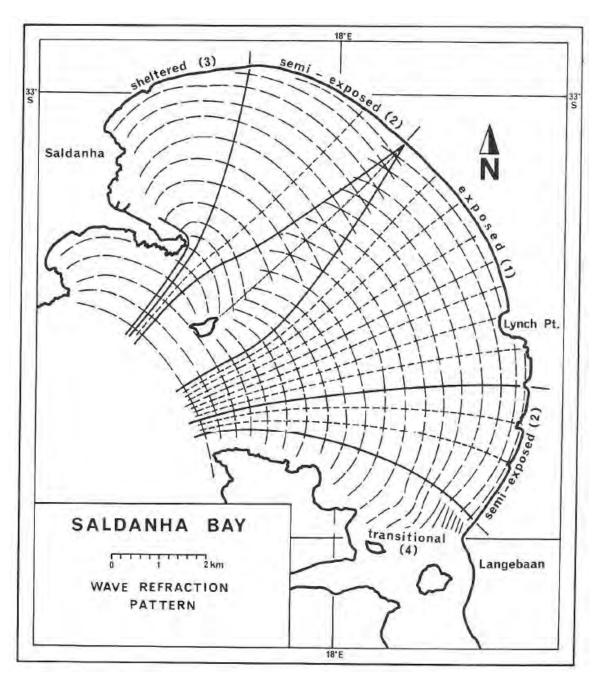
Figure 4.6. Predicted wave field at Saldanha showing wave height and direction. Source: Flemming (1977).
