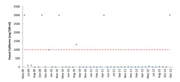
Figure 3.28. Monthly trends in the numbers of Faecal Coliforms in effluent released from the Langebaan WWTW, June 2009 - December 2012. Allowable limits as specified in terms of a General Authorisation under the National Water Act 1998 are represented by the red line.
