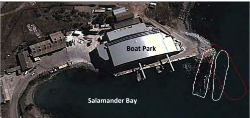
Figure 3.13. Bird's eye view image of Salamander Bay showing the existing boat park, the two shipwrecks (white) and the site of the proposed breakwater (red). The breakwater may either be positioned A) on the outside of the two shipwrecks, or B) on top of sections of the shipwrecks.
