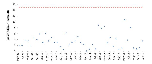
Figure 3.32. Monthly trends in the concentration of Nitrate Nitrogen in effluent from Langebaan WWTW, June 2009 - December 2012. Allowable limits as specified in terms of a General Authorisation under the National Water Act 1998 are represented by the red line.
