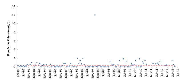
Figure 3.26. Monthly trends in Free Active Chlorine for effluent released from the Saldanha WWTW Apr 2003-December 2012. Allowable limits as specified in terms of a General Authorisation under the National Water Act 1998 are represented by the red line.
