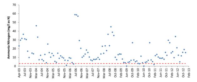
Figure 3.23. Monthly trends in Ammonia Nitrogen for effluent released from the Saldanha WWTW Apr 2003-December 2012. Allowable limits as specified in terms of a General Authorisation under the National Water Act 1998 are represented by the red line.
