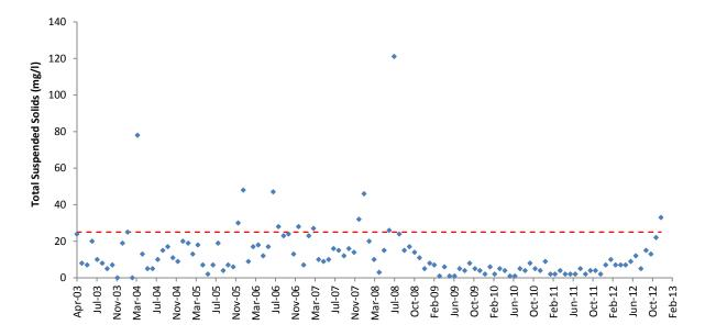
Figure 3.21. Monthly trends in the numbers of Total Suspended Solids in effluent released from the Saldanha WWTW, April 2003 - December 2012. Allowable limits as specified in terms of a General Authorisation under the National Water Act 1998 are represented by the dashed red line.
