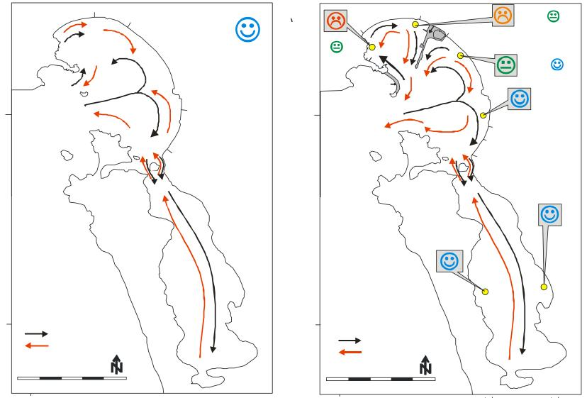
Figure 4.5. Schematic representation of the surface currents and circulation of Saldanha Bay (A) prior to the harbour development (Pre-1973) and (B) after construction of the causeway and iron-ore terminal (Present). (Adapted from Shannon and Stander 1977 and Weeks et al. 1991a)
