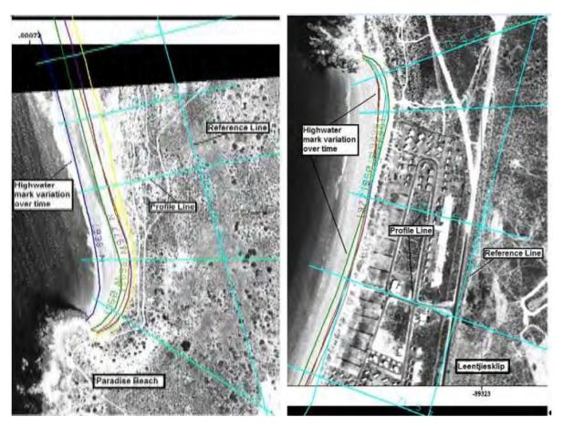
Figure 5.5. Transect (profile) lines (in light blue) used by WSP Africa Coastal Engineers (2010b) to assess long-term changes in the shoreline at Paradise Beach (left) and Leentjiesklip (right) in Saldanha. The high water mark determined from each historical photograph is also shown in dark blue (1938), dark green (1960), purple (1977), light blue (1988), light green (1989) and yellow (2007). Source: WSP Africa Coastal Engineers (2010b).
