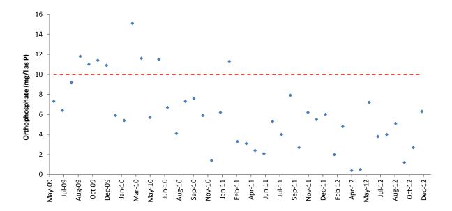
Figure 3.33. Monthly trends in the concentration of Orthophosphate in effluent from Langebaan WWTW, June 2009 - December 2012. Allowable limits as specified in terms of a General Authorisation under the National Water Act 1998 are represented by the red line.
