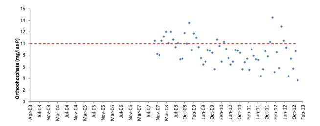
Figure 3.25. Monthly trends in water quality parameters Orthophosphate for effluent released from the Saldanha WWTW Apr 2003-December 2012. Allowable limits as specified in terms of a General Authorisation under the National Water Act 1998 are represented by the red line.
