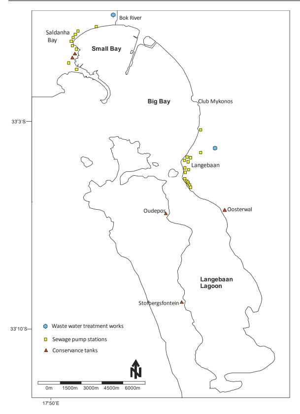
Figure 3.18. Location of waste water treatment works, sewage pump stations and conservancy tanks in Saldanha and Langebaan area (2011).
