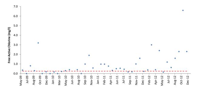
Figure 3.34. Monthly trends in the concentration of Free Active Chlorine in effluent from Langebaan WWTW, June 2009 - December 2012. Allowable limits as specified in terms of a General Authorisation under the National Water Act 1998 are represented by the red line.
