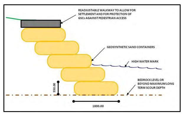
Figure 5.13. Design proposal 1 for the proposed Melck Street walkway: Geosynthetic Sand Container wall. Source: Common Ground Consulting (2013b).
