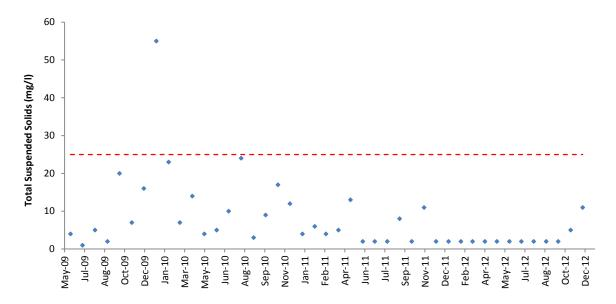
Figure 3.29. Monthly trends in Total Suspended Solids in effluent released from the Langebaan WWTW, June 2009 - December 2012. Allowable limits as specified in terms of a General Authorisation under the National Water Act 1998 are represented by the red line.
