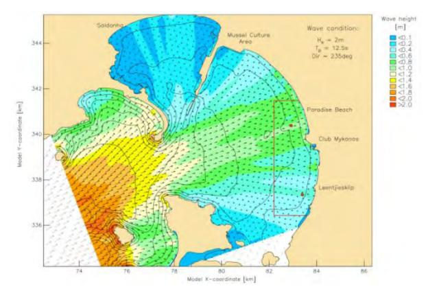
Figure 4.7. Predicted wave field at Saldanha showing wave height and direction. Source: WSP Africa Coastal Engineers (2010).
