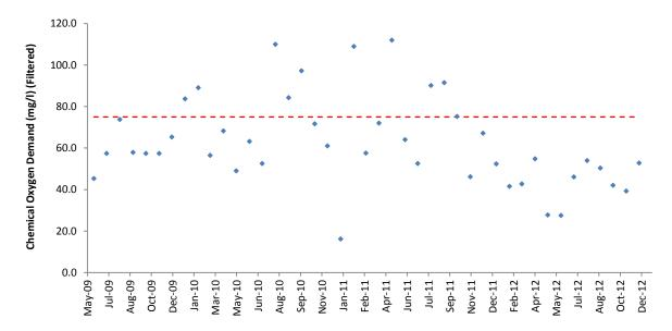
Figure 3.30. Monthly trends in Chemical Oxygen Demand (filtered) in effluent released from the Langebaan WWTW, June 2009-December 2012. Allowable limits as specified in terms of a General Authorisation under the National Water Act 1998 are represented by the red line.
