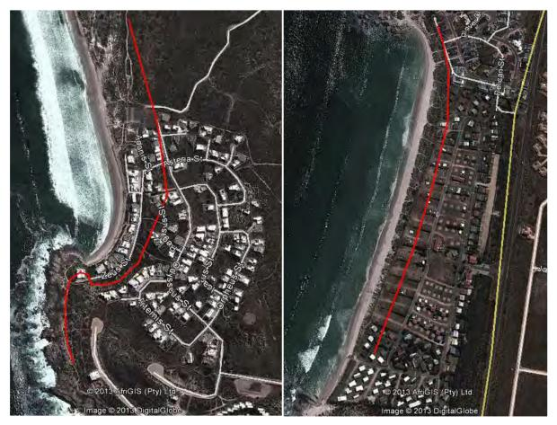
Figure 5.21. Configuration of development setback lines for Paradise Beach (left) and Leentjiesklip (right) as proposed by WSP Africa Coastal Engineers (2010b).
