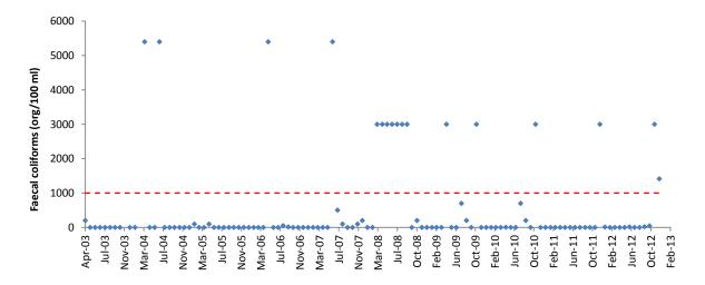
Figure 3.20. Monthly trends in the numbers of Faecal Coliforms in effluent released from the Saldanha WWTW, April 2003 - December 2012. Allowable limits as specified in terms of a General Authorisation under the National Water Act 1998 are represented by the dashed red line.
