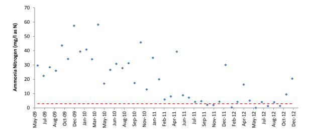
Figure 3.31. Monthly trends in the concentration of Ammonia Nitrate in effluent from Langebaan WWTW, June 2009 - December 2012. Allowable limits as specified in terms of a General Authorisation under the National Water Act 1998 are represented by the red line.
