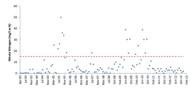
Figure 3.24. Monthly trends in Nitrate Nitrogen for effluent released from the Saldanha WWTW Apr 2003 - December 2012. Allowable limits as specified in terms of a General Authorisation under the National Water Act 1998 are represented by the red line.
