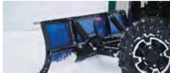
BACK DRAG MODE ALLOWS FOR PULLING SNOW AWAY FROM BUILDINGS
