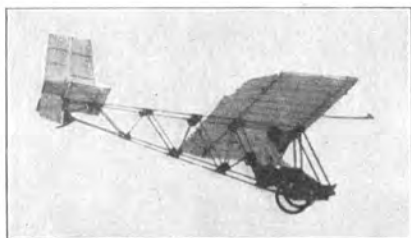
Allen A.E.S. I (1922) E: E. Allen, E. P. Warner, New-York; A: Aeronautical Engineering Society, New-York. S: 1; St: Schw.; Bst: H; P: Martin. — l = 4,50 m; b = 7,50 m; t = 1,50 m; b/t = 1:5,0 ; F = 11,20 m 2 ; Gr = 34,00 kg; Gz = 70,00 kg; G = 104,00 kg; G/F = 9,40 kg/m 2 .
