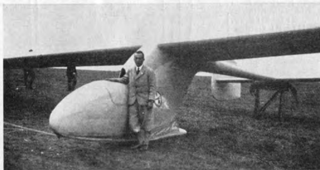
Kupper Ku 4 (1930) E: A. Kupper, Dessau; A: Segelflugzeugbau, Kassel S: 1; St: Schw., Fl.; Bst: H; l = 8,90; h = 2,70 m; b = 30,00 m; t = 1,90; F = 34,97 m 2 ; Hr = 1,29 m 2 ; Hf = 2,03 m 2 ; Sr = 2×0,89 m 2 ; Sf = 2×1,23 m 2 ; Qr = 2×9,4 m 2 ; Tg = 240,00 kg; Lg = 25,00 kg; Rg = 65,00 kg; Gr = 330,00 kg; Gz = 83,00 kg; G = 413,00 kg; G/F = 11,8 kg/m 2 .
