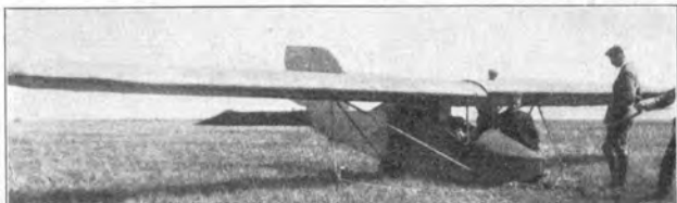
Dresden „Doris“ (1922) E: H. Muttray, R. Seifert, Dresden; A: Flugtechn. Verein, Dresden. S: 1; St: Fl.; Bst: H; P: Göttingen 441; Gwkl = 1 : 14,6. - l = 4,93 m; h = 1,28 m; b = 12,20 m; t = 1,35 m; b/t = 1 : 9,5; F = 15,50 m 2 ; Hr = 1,90 m 2 ; Sfl = 0,66 m 2 ; Sr = 0,55 m 2 ; Tg = 65,20 kg; Lg = 8,20 kg; Rg = 45,10 kg; Gr = 118,50 kg; Gz = 75,00 kg; G = 193,50 kg; G/F = 12,50 kg/m 2 .
