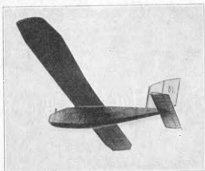
Messerschmitt S 14 (1923) E: W. Messerschmitt, Bamberg; A: W. Messerschmitt, Bamberg. S: 1; St: Fl.; Bst: H; P: Göttingen 535. — B.-L.: H: 303 m. — l = 5,40 m; h = 1,35 m; b = 14,00 m; t = 1,35 m; b/t = 1:10,3; F = 17,50 m 2 ; Hr = 2,40 m 2 ; Sfl = 0,70 m 2 ; Sr = 0,80 m 2 ; Gr = 105,00 kg; Gz = 70,00 kg; G = 175,00 kg; G/F = 9,60 kg/m 2 .
