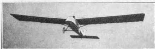
Nordman (1924) E: Nordman, Flush; A: Nordman, Flush. S: 1; St: Schw.; Bst: H; P: U. S. A. TS 10. — l = 5,80 m; h = 1,80 m; b = 12,20 m; t = 1,40 m; b/t = 1:8,7 ; F = 17,50 m 2 ; Gr = 90,00 kg; Gz = 70,00 kg; G = 160,00 kg; G/F = 8,80 kg/m 2 .
