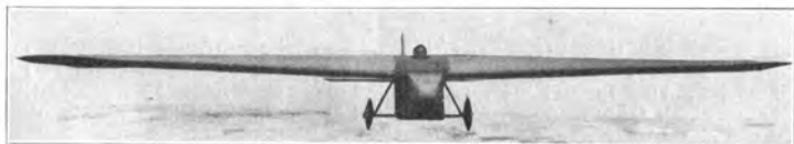
Dewoitine D 1 (1922) E: E. Dewoitine, Toulouse. A: E. Dewoitine, Toulouse; S: 1; St: Schw.; Bst: H; P: Göttingen 430. — B.-L.: D: 8:36:56 h; H: 546 m. — l = 4,90 m; b = 11,30 m; t = 1,13 m; b/t = 1 : 10,0; F = 11,50 m 2 ; Gr = 110,00 kg; Gz = 60,00 kg; G = 170,00 kg; G/F = 14,70 kg/m 2 .
