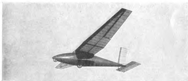
Hannover H 6 „Pelikan“ (1923) E: A. Pröll, W. Günther, W. Mertens, Meyer, Hannover; A: Hannoversche Waggonfabrik, A.-G., Hannover. S: 1; St: Schw; Bst: H; P: Göttingen 396; vg = 12,90 m/s; Gwkl = 1:28 ; vs = 0,46 m/s. — B.-L.: D: 0:30:0 h. — l = 5,26 m; h = 1,25 m; b = 15,00 m; t = 1,00 m; b/t = 1:15,0; F = 15,00 m 2 ; Hr = 1,80 m 2 ; Sr = 0,66 m 2 ; Tg = 45,00 kg; Lg = 4,50 kg; Rg = 25,50 kg; Gr = 75,00 kg; Gz = 70,00 kg; G = 145,00 kg; G/F = 9,50 kg/m 2 .
