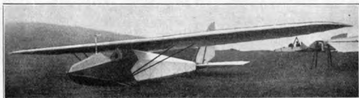
Spalinger S 9 (1927) E: J. Spalinger, Schwamendingen; A: J. Spalinger, Schwamendingen. S: 1; St: Schw.; Bst: H; P: Göttingen 358; l = 5,20 m; b = 12,50 m; F = 13,40 m 2 ; Gr = 95,00 kg; Gz = 70,00 kg; G = 165,00 kg; G/F = 12,30 kg/m 2 .
