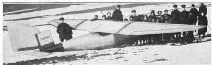
Espenlaub E 5 (1923) E: G. Espenlaub, Wasserkuppe; A: G. Espenlaub, Wasserkuppe. S: 1; St: Schw.; Bst: H. — l = 5,00 m; h = 1,50 m; b = 12,00 m; t = 1,20 m; b/t = 1:15,0 ; F = 14,00 m 2 ; Hr = 2,20 m 2 ; Sfl = 0,45 m 2 ; Sr = 0,70 m 2 ; Gr = 86,00 m; Gz = 70,00 kg; G = 156,00 kg; G/F = 10,30 kg/m 2 .
