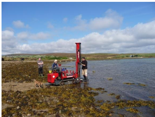
Figure 26: Coring to sample submerged peat deposits at Mill Bay, Hoy ©Rising Tide
