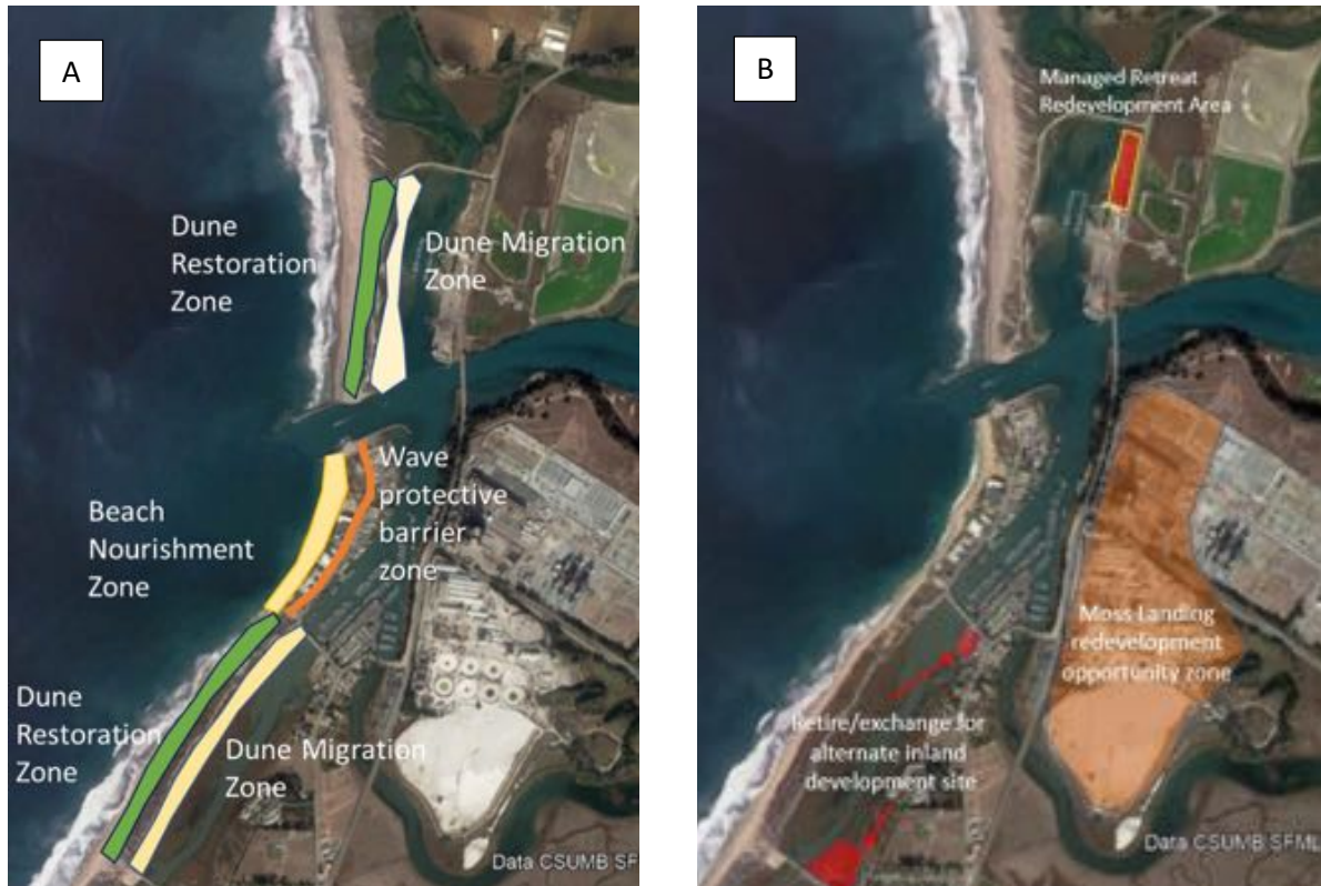
Figure 14. Maps of (A) areas for recommended coastal dune and beach management zones to increase resiliency of natural dune barrier and work with ML island property owners to develop a storm surge barrier into new and existing development and (B) possible areas in harbor ownership where development opportunities could be retired and exchanged for development in areas resilient to 2060 hazards (Moss Landing community redevelopment opportunity zone also noted although outside of harbor district control).
