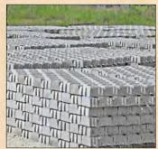
SHOREBLOCK\* SD blocks of different heights and weights can be assembled to provide a castellated cover layer for a higher coefficient of hydraulic friction or improved wave energy absorption and retention.
