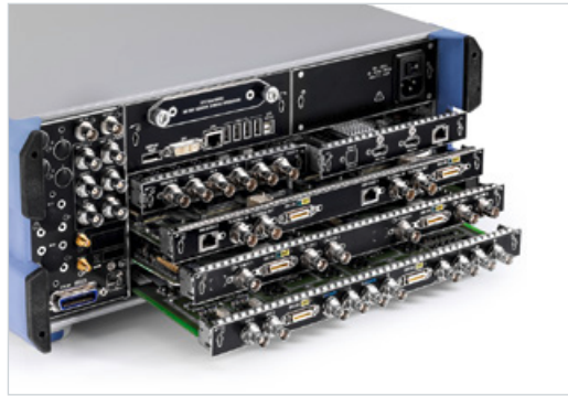
Due to its modular design, the R&S®BTC hardware can be ideally adapted to different measurement tasks.
