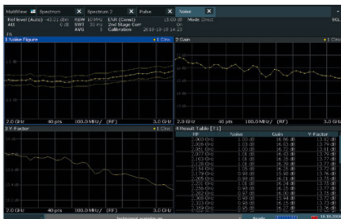
Fig. 1: Noise figure and gain measurement with R&S®FSx-K30 application firmware. In addition to the result table and the noise figure traces, the calculated gain and Y factor uncertainty can also be displayed.
