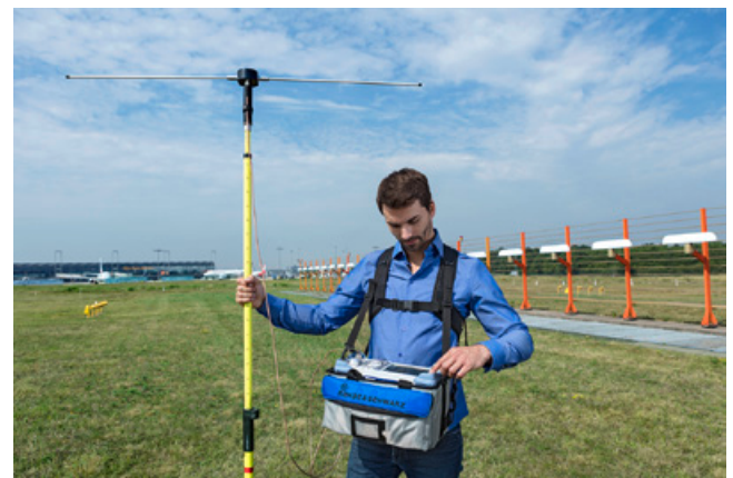
ILS measurements with R&S®EVS-Z3 ILS/VOR test antenna
