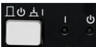
Figure 2-4: Standby switch and LEDs
