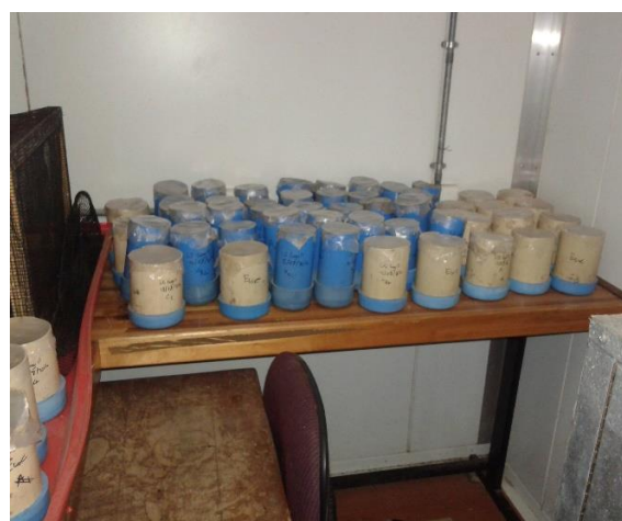
Figure 3.3. Photographs of the soil-cores placed in an incubation room. The PVC soil-cores were sealed with parafilm as to prevent any rapid drying of the soil. The soil-cores were labelled with the date of treatment and the type of treatment.
