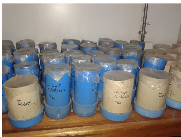
Figure 3.3. Photographs of the soil-cores placed in an incubation room. The PVC soil-cores were sealed with parafilm as to prevent any rapid drying of the soil. The soil-cores were labelled with the date of treatment and the type of treatment.
