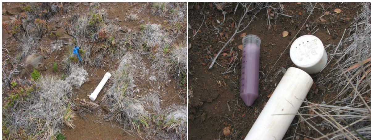
Figure 1. Bait station design chosen for the experimental plots. The panel on the left shows placement of a bait station in the field, while the panel on the right shows a close-up view of one endcap (removed) with the four entrance holes, as well as an internal bait tube containing bait stoppered with a cotton ball.
