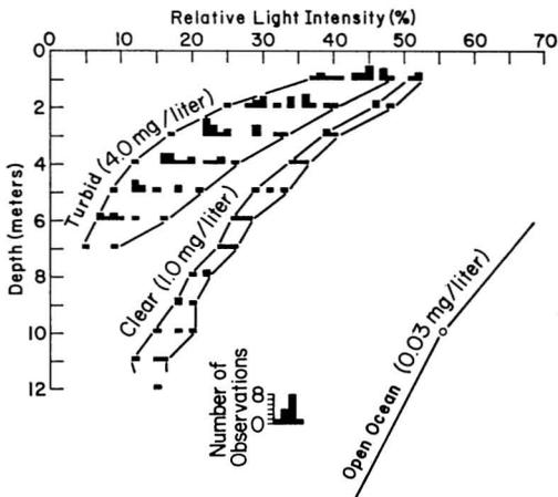
FIG. 8. Relative light intensity versus depth in the clear-water area, the turbid-water area, and the open ocean. The suspended load (e.g., 4.0 mg/liter) is the average weight of suspended  $\text{CaCO}_3$  in each of the three areas. The relative light intensity in the open ocean is for an area off Hawaii.
