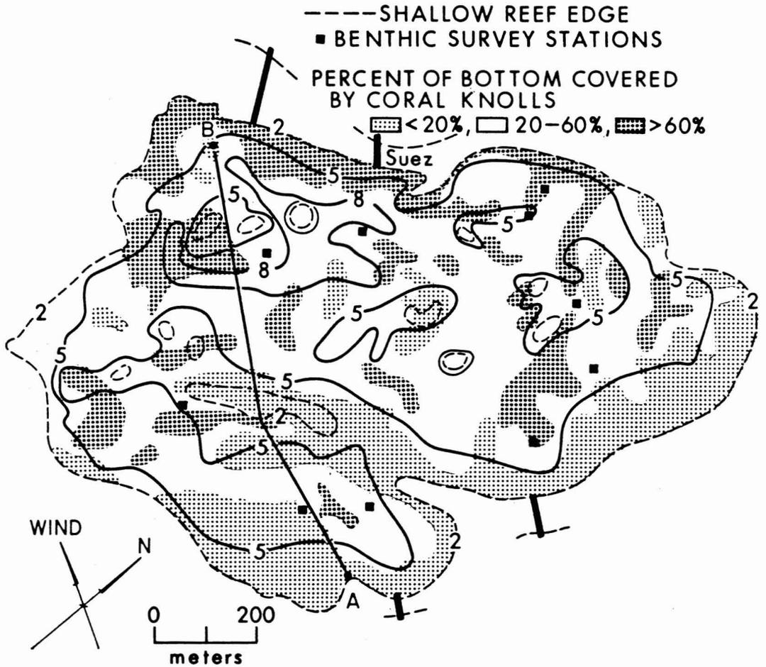
FIG. 4. Bathymetry and coral knoll abundance in the turbid-water pond. The line A-B is the profile shown in Figure 3. Contour interval is 3 m.
