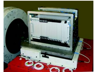
Shock and vibration resistant in all three axial directions
