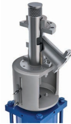
SchuF Ram/Piston Injection Valve with pneumatic linear actuator and hollow piston, which can feature up to 2000 holes for high flow rates
