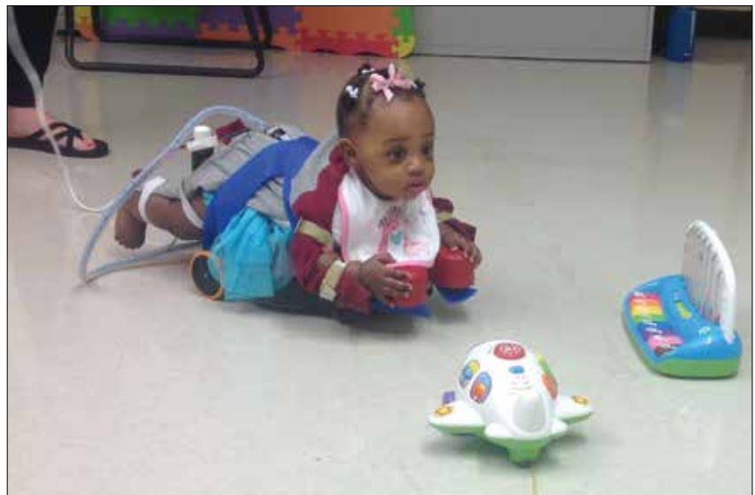
The motorised SIPPC has sensors that respond to a baby's kicks and weight shifts. The device rewards the baby with an extra boost. Photo: University of Oklahoma Health Sciences Center.
