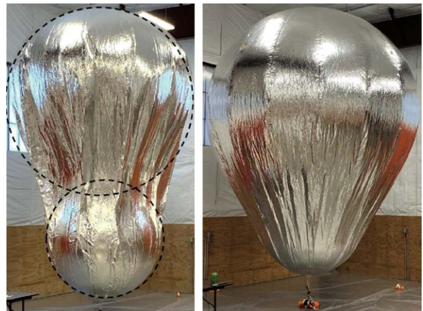
Figure 6: JPL/Near Space Corporation 4 m sub-scale variable altitude balloon (2020), illustrating the volume expansion required for changing altitude. [Izraelevitz, J., Pauken, M., Elder, T., Carlson, K., Lachenmeier, T.I.M., Baines, K., Cutts, J.A. and Hall, J.L.. “Pumped-Helium Aerobots for Venus: Technology Progress and Mission Concepts. 2020, December”. In AGU Fall Meeting 2020. AGU.]
