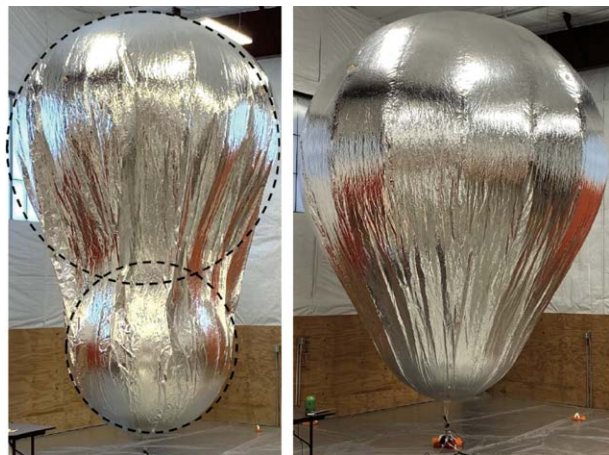
Figure A-9: JPL/Near Space Corporation 4 m sub-scale variable altitude balloon (2020), illustrating the volume expansion required for changing altitude. [Izraelevitz, J., Pauken, M., Elder, T., Carlson, K., Lachenmeier, T.I.M., Baines, K., Cutts, J.A. and Hall, J.L. “Pumped-Helium Aerobots for Venus: Technology Progress and Mission Concepts. 2020, December”. In AGU Fall Meeting 2020. AGU.]
