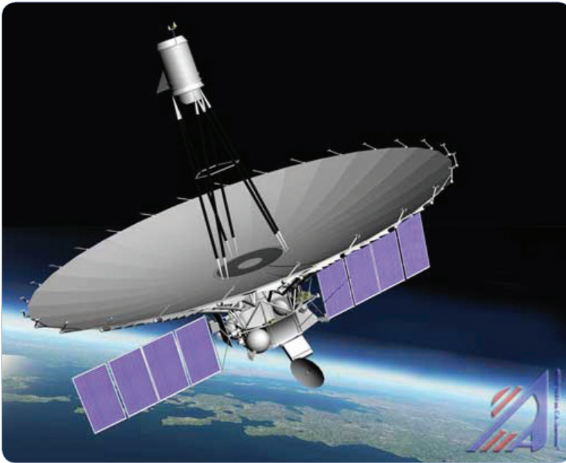
Artist rendering of the orbiting RadioAstron satellite, the farthest element in an array of radio antennas that combine to form the highest resolution instrument in all of astronomy. Credit: Lavochkin Association.
