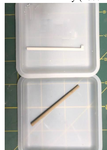
Figure 4: YSZ (top) and alumina (bottom) nozzle reactors created with our ceramic micro-reactor manufacturing process.
