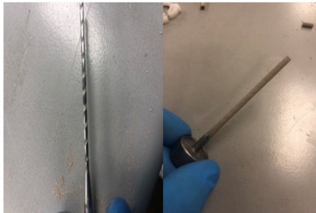
Figure 5: (Left) Image of the stainless-steel mandrel produced using DMLS. (Right) Image of the silicon carbide compact post isostatic pressing
