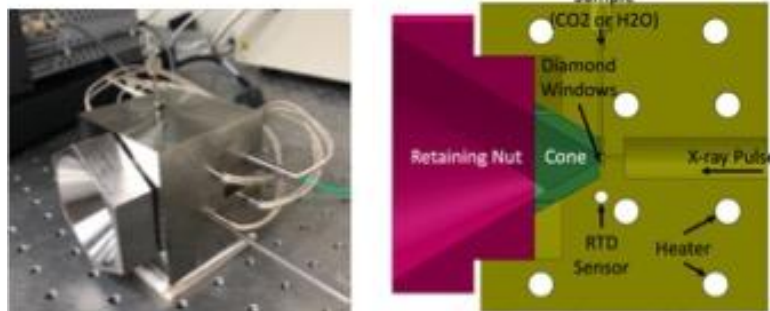
Figure 1: High-pressure cell with cartridge heaters and temperature sensor (left) and cross section through pressure cell (right).
