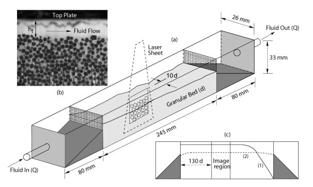
**Figure 1:** (a) Schematic diagram of our experimental apparatus for exploring grain-scale motions at the threshold for erosion. (b) Sample image of the refractive index matched beads in a plane away from the side walls. (c) Side view of the experimental apparatus.
