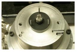
Fig. 1 Pre-shaped Kalrez membrane and mini-bending jig
