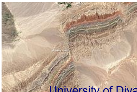
Fig.(5.1) Shows oblique left lateral strike slip faults and en echelon right lateral active faults.
