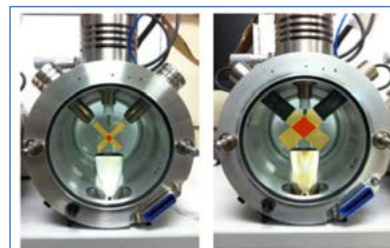
Figure 4: SCIEX TurboV source(left) and SCIEX IonDrive source(right) have different ion source temperatures that are optimal for each model.
