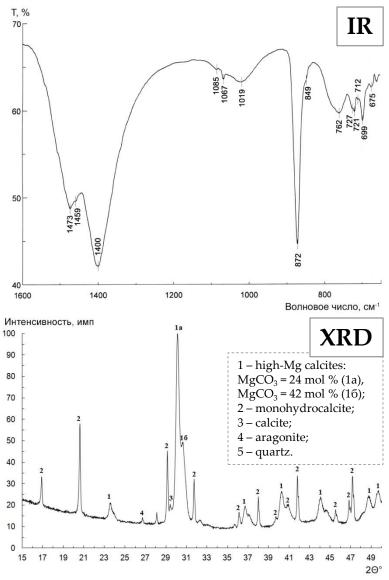
The predominantly carbonate composition of microbialites was revealed using infrared spectroscopy (IR) and X-ray diffractometry (XRD). Carbonates are represented mainly by high-magnesium calcites and monohydrocalcite. Calcite and aragonite are found in minor quantities. In addition, a small amount of silicates and amorphous hydromagnesite are found.
