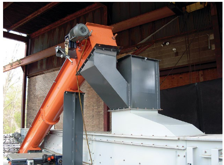
Inclined Super-Flo Drag Conveyor discharging materials into a hopper/pan-feeder inlet on a Super-Flo XL Flat Bottom Drag Conveyor.
