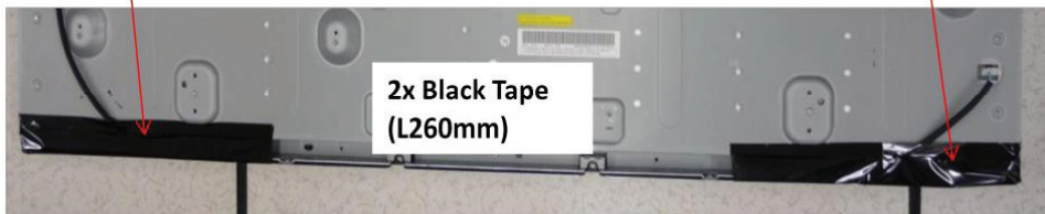
Figure 4-10 Light leakage solution (only for 37" model)
