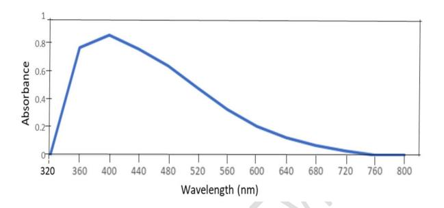
Fig. 2 UV–Vis spectrum of the colloidal solution of *Pleurotus ostreatus* extract and AgNO<sub>3</sub> showing maximum absorption at 400 nm due to the presence of AgNPs
