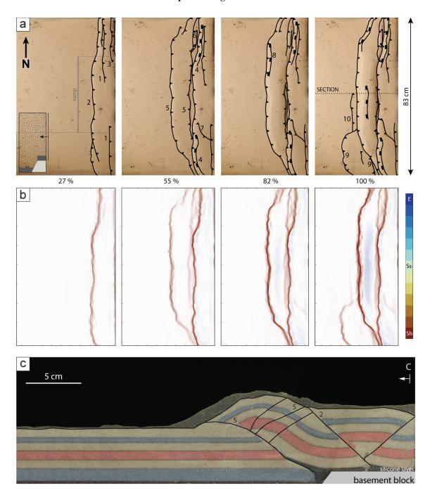
**Figure 11.** Modelling results of model C, showing (a) top views at 27 %, 55 %, 82 %, and 100 % of total shortening. (b) Analysis of cumulative (surficial) strain showing strain types of model C. Colours show areas of extension (E), strike-slip movement (Ss), and shortening (Sh). The inset in the first top-view photograph shows the modelling setup in cross-sectional view. Panel (c) shows a side view at 100 % of total shortening. Numbers show the sequence of fault formation.
