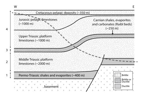
**Figure 6.** Schematic diagram showing the geological set-up of the eastern margin of the Achental basin, prior to inversion. The dashed line represents the trace of the Achental thrust. Lithologies are marked brittle or ductile depending on their mechanical properties. Numbers refer to layers in Fig. 3.
