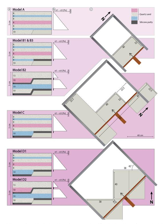
**Figure 7.** Modelling set-up for model series A–D. (a) Layering sequences show differently coloured layers of quartz sand and silicone putty with their respective thickness (in mm). The total thickness of the layering sequence was 5 cm. (b) Strength envelopes show the strength (in Pa) of different modelling materials. (c) Basal plate set-ups show the basal plate size (in cm).
