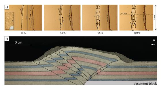
**Figure 8.** Modelling results of model A, showing (a) top views at 25, 50, 75, and 100% of total shortening and a (b) side view at 100% of total shortening. The location of the section is marked in (a). Numbers show sequences of fault formation. The inset in the first top view photograph shows the modelling setup in cross-sectional view.
