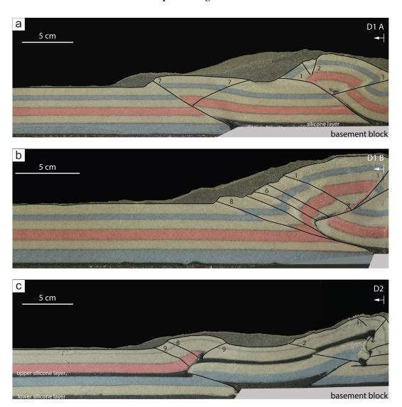
Figure 13. Side views of models (a, b) D1 and (c) D2 at 100 % of total shortening. Numbers show the sequence of fault formation.
