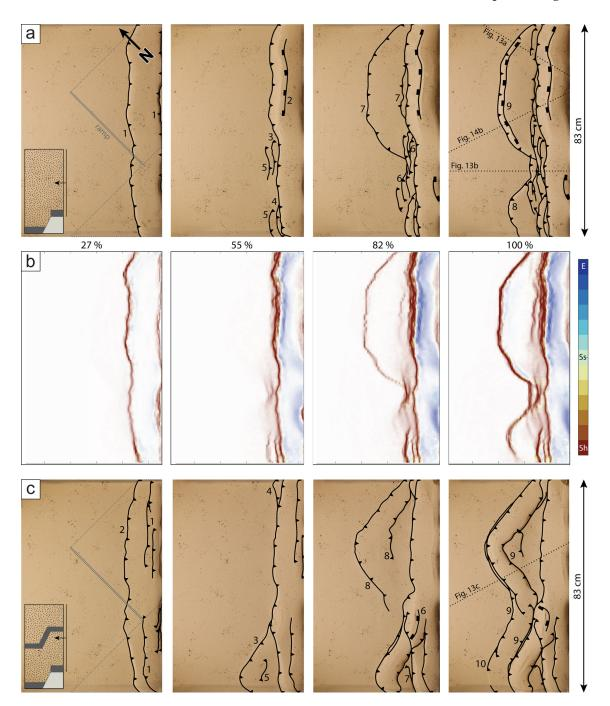
**Figure 12.** Top view of models (a) D1 and (c) D2 at 27 %, 55 %, 82 %, and 100 % of total shortening. Numbers show the sequence of fault formation. The insets in the first top-view photographs show the modelling setups in cross-sectional view. The PIV strain type analysis of model (b) D1 shows areas of extension (E), strike-slip movement (Ss), and shortening (Sh).
