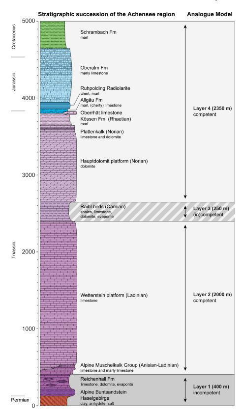
**Figure 3.** Stratigraphic overview of the Permian–Cretaceous sedimentary succession of the Karwendel thrust sheet in the Achensee area, modified after Kilian et al. (2021). Various sedimentary strata have been assigned to different incompetent and competent layers (1–4) in the analogue model set-up (see also Fig. 6). The Raibl beds were modelled as incompetent or competent, depending on the specific model. Kilian et al. (2021) discuss the rheological behaviour of the Raibl beds in more detail.
