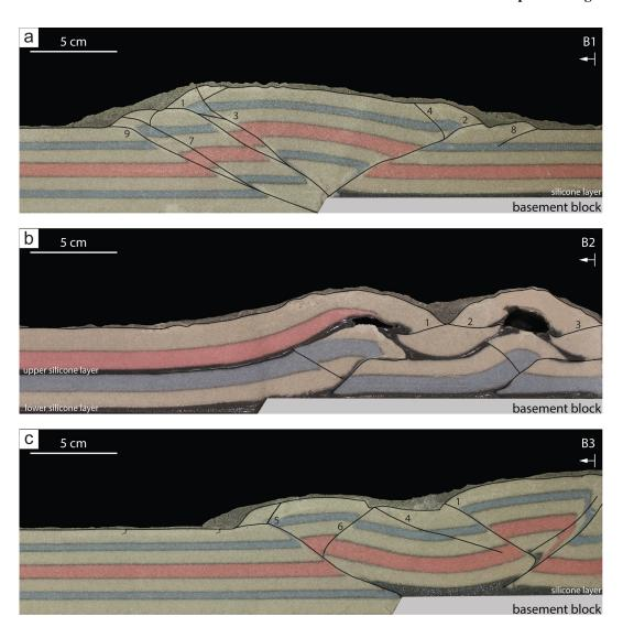
Figure 10. Side views of models (a) B1, (b) B2, and (c) B3 at 100 % of total shortening. Locations of sections are marked in Fig. 9. Numbers show the sequence of fault formation.
