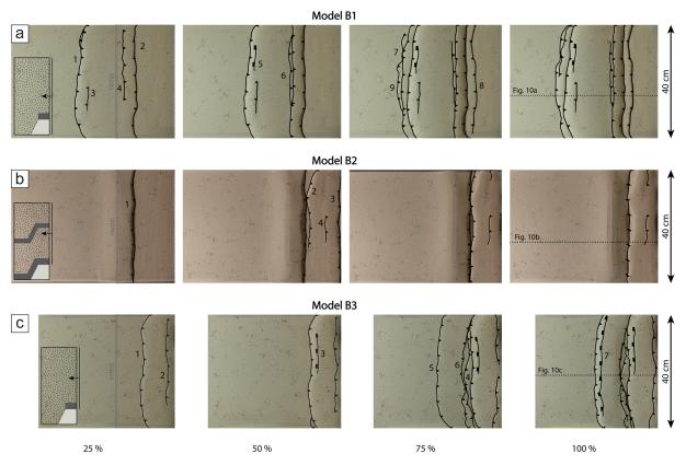
**Figure 9.** Top views of models (a) B1, (b) B2, and (c) B3 at 25 %, 50 %, 75 %, and 100 % of total shortening. Locations of sections are indicated (dotted lines). Numbers show the sequence of fault formation. The insets in the first top view photographs show the modelling setups in cross-sectional view.
