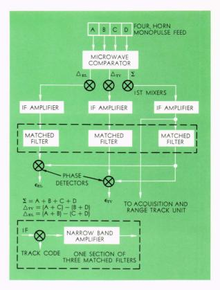
Fig. 5-Monopulse angle error processing system.
