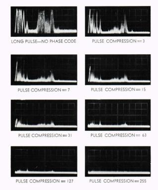
Fig. 8—Detected video out of digital pulse compressor on rainstorm (100  $\mu$ sec/cm common to all).
