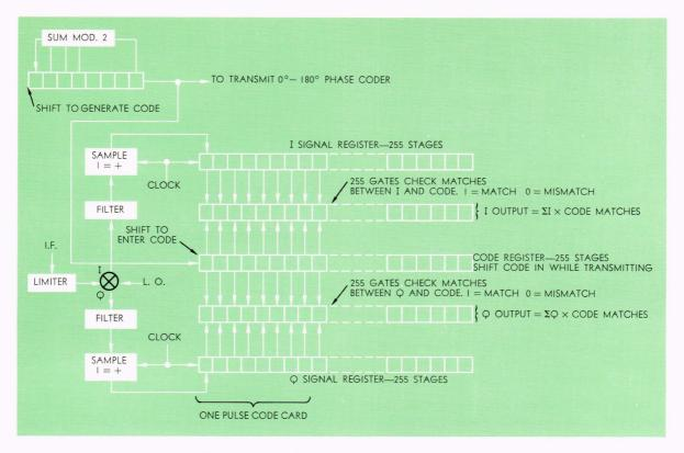
Fig. 2-Block diagram of digital compressor.
