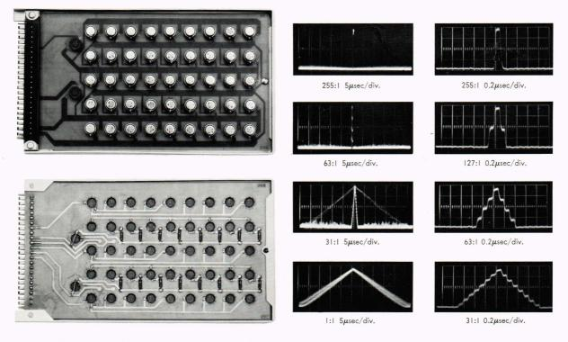
Fig. 3—Eight-stage digital compression card, fourlayer board.
