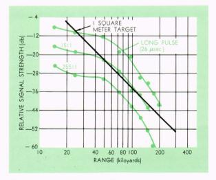
Fig. 9—Snow clutter profiles for three compression ratios. Condition dry snow ( $\sim 1 \text{ mm/hour water}$  equivalent).
