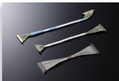
Micro Flex Coaxial (MFCX) Cable MFCX cable has an extremely small outer diameter ranging from 0.20 to 0.35 mm. This cable is mainly used in the hinge connection area between the motherboard and LCD of a laptop PC or mobile-phone. Double-shielded structure is also available to enhance noise immunity.
