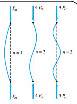
**FIG. 10.4** First three buckling mode shapes of a simply supported column.
