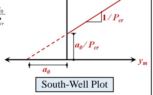
The values of  $y_m / P$  and  $y_m$  are plotted from a column test then these variables can be related by a straight line.
