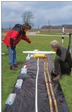
Installation of a 3-Channel CMT System with bentonite and sand cartridges. Three zones were monitored over a 20 ft (6 m) depth. The installation was completed in glacial till at the University of Waterloo, Ontario Canada.
