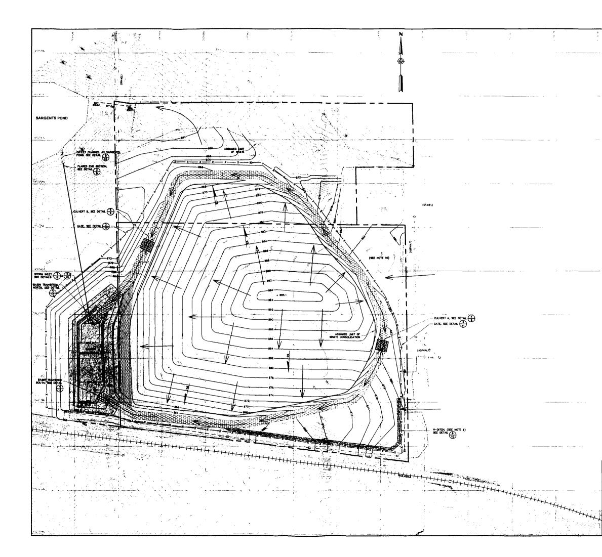
LEGEND ASSUMED UNIT OF WASTE FORSTING OROLIND SUPPACE CONTOLIN (1 FT) BLBLONG FOOTPRE POWER LINE GAS LINE (SEE NOTE 7 ++++++++ RAUROAD ÷-UTILITY POLE - x- x- x- proposed fenceline, see detail (1)  $\leftarrow$ STURMWATER FLOW DIRECTION BASIN SECTION, SEE DETAIL (4) & (5) PERMETER CHANNEL, SEE DETALS CAP TO BASH TRANSITION, SEE DETAL V DITCH, SEE DETAL Channel crossing, see details  $\begin{pmatrix} 4 \\ 1 \end{pmatrix} = \begin{pmatrix} 5 \\ 1 \end{pmatrix}$
