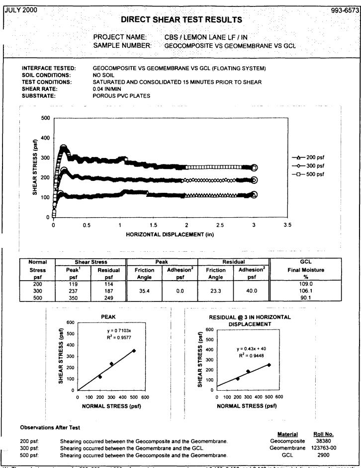
(1) The peak shear stresses for 200, 300, and 500 psf normal stresses were chosen at 0.103, 0.158, and 0.148 in horizontal displacements, respective which may not show the maximum shear stress.
